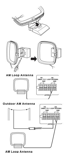
**Note:** For the best results, use 75-ohm coaxial cable to connect an outdoor antenna to the receiver.
